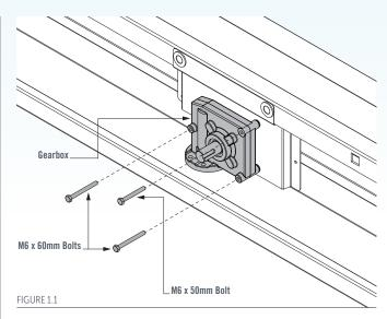
Use the Gearbox as a template to mark the positions for the two front eyelet mounting holes. Mark around the base flange of the Gearbox to help with the hole positioning in the next step (Figure 1.2).
