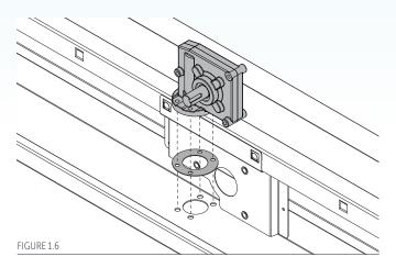
Fit together the Eyelet Assembly by sliding the Eyelet into the Shoulder Washer, and then the Shoulder Washer into the Eyelet Locating Flange. Ensure that the Shoulder Washer is fully seated in the Locating Flange. The Gearbox Coupling will fit onto the D-Shaft on the Eyelet (Figure 1.7).
