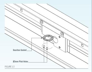
Carefully drill pilot holes through the gutter from above using a Ø3mm drill bit.
