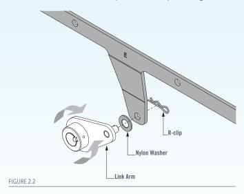
Insert the Crank Handle into the Eyelet and open and close the louvres to pull the Link Arm into alignment. Tighten the grub screw on the Link Arm using a 2mm allen key (Figure 2.3).
