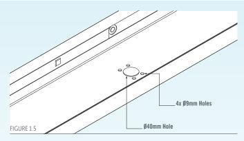
Remove any burrs using a file and brush out any swarf in the gutter to avoid corrosion.
