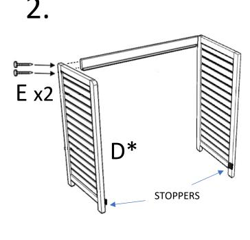
$<sup>{}^{*}\</sup>text{Each 'D'}$  panel has a wooden stopper on one side near the base, this is to face **inwards.**
