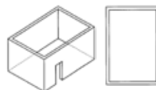
Figure 1: Enclosure with walls on all sides but no overhead cover
