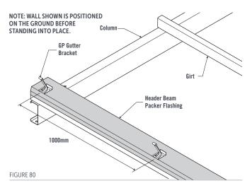
Stand the wall frame in the footing holes, and temporarily brace it with props.
