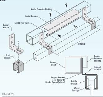
Rivet the sliding door flashing to the header extension flashing, then pan fix the Superdek® gable end wall sheets to the open gable end with 10x16mm self drilling screws.
