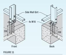
Each stirrup is fixed to the column with four bolts and into the concrete perimeter beam with four M16 threaded rods with chemical injection to set anchors. Threaded rods will need to be cut to the required length before embedding into the concrete.
