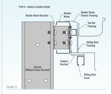
Fix the gutter brackets to the header beam packer flashing at approximately 1000mm centres with rivets.
