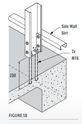
Embed the rod a minimum of 250mm into the slab.
