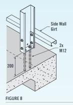
Embed the rod a minimum of 200mm into the slab.
