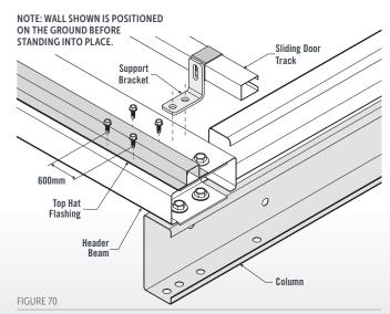
Rivet the sliding door flashing to the packer flashing at 300mm centres. Align the sliding door flashing with the bottom face of the header beam packer flashing, see Figure 70.
