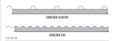
Note, Cooldek sheets are supplied with the top sheet 60mm longer than the insulating foam core and under sheet to allow for the cutback flashing and gutter to be attached. Ensure this end of the sheet is installed at the Eaves of the shed
