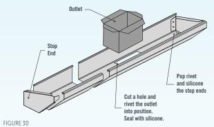
Fix the gutter to the crest of Superdek sheets, or to the gutter attachment flashing if Hiland Tray is used. Allow for a slight fall towards the downpipe end so the water can flow freely.
