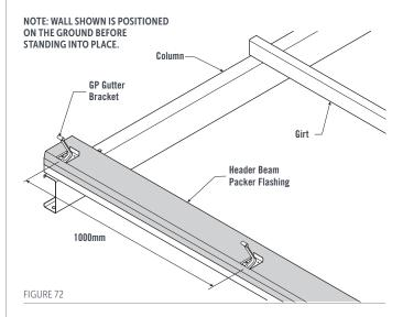
Stand the wall frame in the footing holes, and temporarily brace it with props.
