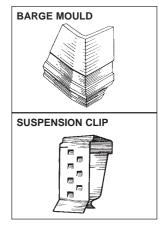
When ordering ensure either Clickform™ or Clickfast® components are clearly specified. Barge moulds should be specified left or right hand when ordering.
