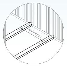
Ensure a maximum distance between Beams of 450mm.
