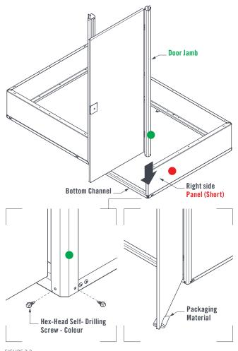
Fasten one coloured Sheetmetal Screw through the Door Jamb and Door Stop and into the Panels (Short) from the inside of the shed.
