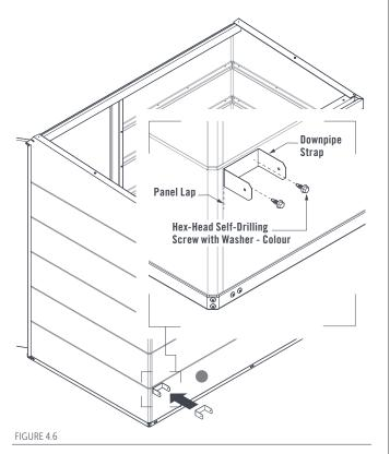
Fit the Downpipe over the Downpipe Outlet and hard against the underside of the Gutter. Fasten the Downpipe to the Downpipe Strap using two Coloured Hex-Head Self-Drilling Screws.
