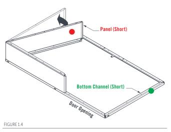
Ensure Panels lap together at corners in the correct manner. The Left Panel fits into the inside of the Front Panel. The Rear Panel fits into the inside of the Side Panels.
