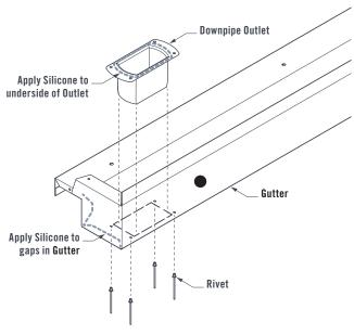
Fit the Gutter over the rear Panel (Long). Ensure the Gutter fits under the Barge Panels.
