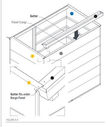
Fasten one coloured Sheetmetal Screw through the Barge Panel and into the **Gutter** at both ends.
