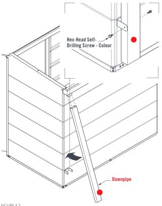
Drill two Ø3.5mm holes through the Downpipe and into the Downpipe Outlet. Rivet the Downpipe to the Downpipe Outlet with two coloured Rivets.
