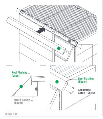
Fasten coloured Hex-Head Self-Drilling Screws with Washers through the top of the Barge Panels at all four corners and middle pilot holes. Fasten a coloured Hex-Head Self-Drilling Screw with Washer through the Door Stop and into the Panel (Short).
