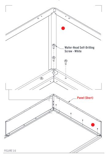
Fit a Panel (Short) to the right side Bottom Channel (Short). Install the panel at an angle (Figure 1.7).
