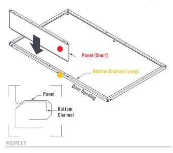
Fasten the Panel (Short) to the Bottom Channel (Long) with four white Wafer-Head Self-Drilling Screws.
