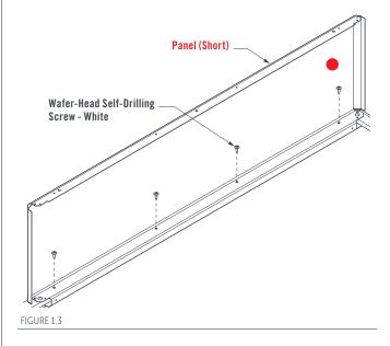
Fit a Panel (Short) to the left side Bottom Channel (Short). Install the Panel (Short) at an angle (Figure 1.4).
