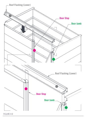
Fasten two coloured Sheetmetal Screws through the Barge Panels and into the Roof Flashing (Lower) at both ends.
