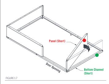
Fasten the Panel (Short) to the Bottom Channel (Short) with four white Wafer-Head Self-Drilling Screws.
