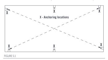
Refer to anchoring locations (Figure 5.1). Using the holes in the Anchor Plates as a guide, drill a hole into the concrete slab through all six Anchor Plates using a 10mm Masonry Drill Bit. Fix all six Anchor Brackets to the concrete slab using six M8x47 Masonry Anchors (Figure 5.2).
