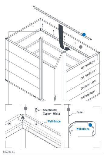
Assemble the remaining Panel layers. Note: For the sixth Panel layer, fit a Barge Panel (Left) and
