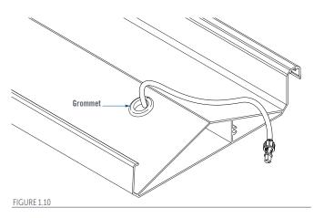
Replace the louvre end cap, then re-install louvres into the frame and reconnect the link rod.
