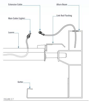
Connect the extension cables to the power supply and to the main cables at each louvre, ensuring the connections are screwed tight (Figure 1.6).
