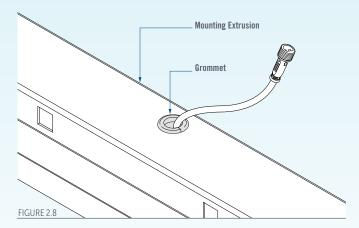
Carefully move the louvres through their full travel and check that the cables don't interfere. Adjust the cable lengths by pushing excess cable into the louvres, Mounting Extrusion, or Allure beam.
