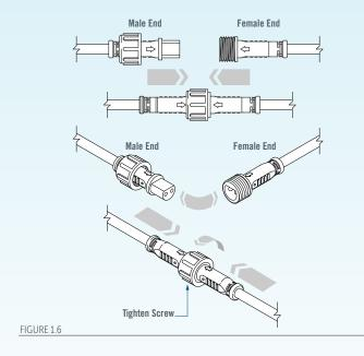
Connect the female cable ends to the light fixtures (Figure 1.6). Apply the supplied heat transfer adhesive all the way around the contact surface of the lights (Figure 1.7).
