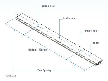
Using a Ø48mm holesaw drill two holes for the lights in the marked positions (Figure 1.2).
