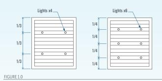
Measure and mark out the position of the lights along the centre line of each louvre. The recommended distance between lights is 1500mm to 2000mm (Figure 1.1). Ensure the spacing from the ends of the louvres to the holes is even at each end.
