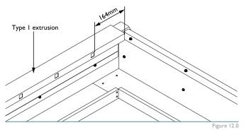
Based on the length of the unit, cut the extrusion so it fits inside the box gutters. Clamp the extrusion to the beam and screw fix with 12x20 self drilling screws at 900mm centres. Repeat this step for the other type of the extrusion on the other side.
