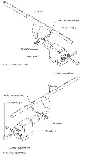
Attach the adjustment bolt to the other end of the actuator with an  $M8 \times 10 \times 20$  shoulder bolt (Figure 15.0). Secure with an M8 washer and lock-nut (do not over tighten the lock nut). Ensure the flat surface on the adjustment bolt faces up.
