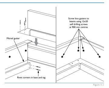
Insert the two remaining box gutters over the mitred ends and screw fix to the framework with 12x20 hex head self drilling screws at 900mm centres. Rivet the corners together through the base of the gutter, and through the folded tag and upright. Silicone all rivet holes and material connections to ensure the gutter is water proofed.
