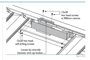
If two link rods are required, for louvre banks over 3m (14 louvres), the link rods will need to be joined using a Link rod joiner. Make sure to join the link rods at the uncut ends.
