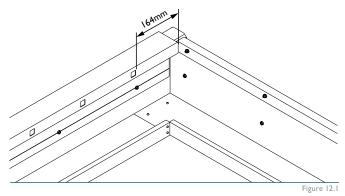
Measure the remaining distance between the Mounting Extrusion edge and box gutter cover at the other end and cut the second extrusion (use the different type) to fit the length. It is important to cut the second extrusion from the correct end, do not cut the end which has the dots (Figure 12.2).
