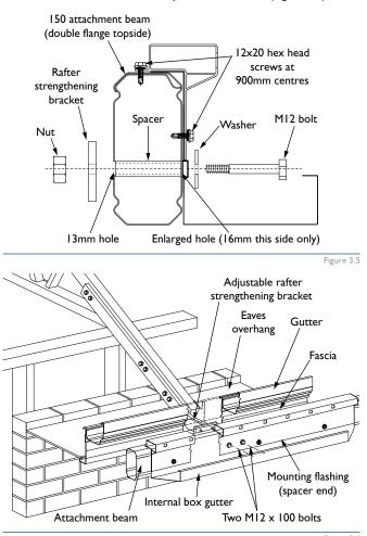
**Note:** Do not over tighten the bolts as this can lead to a visible indentation due to the high gloss nature of the material.
