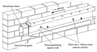
**Note:** Anchor size and spacing may not be suitable for hollow block construction, refer to Stratco for further advice.
