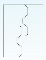
Ensure the top Panel is lapped over the bottom Panel.
