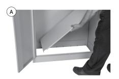
Place the Floor Panel into position with the cutouts facing the front.
