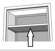
Screw the top panel to the inside of the cabinet as indicated by the arrows
