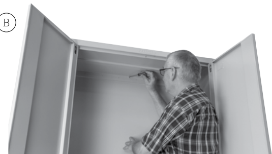
Fasten to the Back Panel with 3 x screws. Then, use a screwdriver to push the 'push-through' slots shown at 'A' into the Front Panel.
