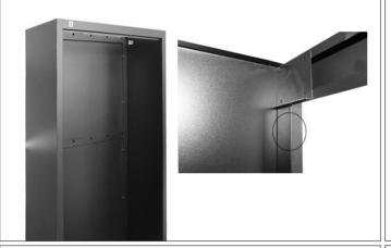
Step 4 Assemble top plate from inside using 6 x M5x12 screws. The screw holes are on front and back rims.
