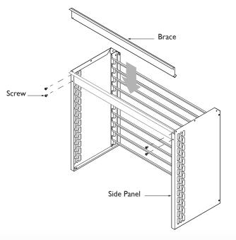
For an accurate fitment, fasten the front-most screws through the Side Panels and into the Top Panel first.
