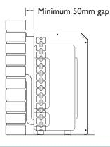
Ensure air-flow gap of at least 50mm between the Side Panels and vented faces of the air conditioner unit.
