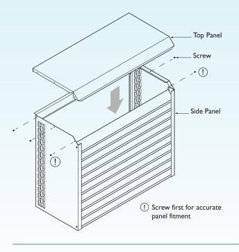
There must be a minimum 50mm gap between the Side Panels and wall. Failing to leave an adequate gap will restrict airflow to the air conditioner unit.
