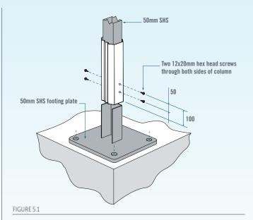
Use construction props or bracing to hold columns in position but do not bolt to the concrete slab at this stage.
