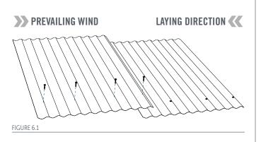
Lift the first sheet into place and push it firmly into the BIP foam in the back channel to weather proof it. Roofing should have a 50mm overhang into the gutter. Check the sheet is square against the back channel and side rafter. At the back channel end, rivet the sheet from underneath through the bottom of the back channel with 3.2mm rivets (Figure 6.2). Seal the rivets with silicone inside the back channel.
