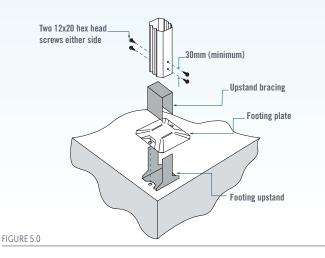
Slide the assembled footing bracket and bracing into the bottom of the column, and fasten with two 12x20 hex head screws either side ensuring the top screws are located at least 15mm from the top of the upstand with screws being a minimum 30mm apart (Figure 5.0).
