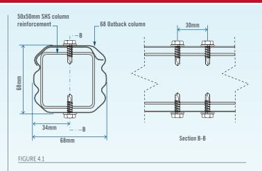
The unfluted faces of the column should be aligned with each face of the post to beam bracket. Fasten the 68 Outback column to the post bracket using two 12x20 hex head screws either side (Figure 4.1).
