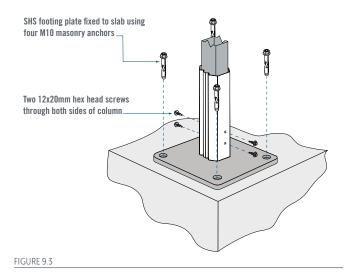
**Note:** Anchors to be installed in accordance with manufacturer's specifications with appropriate concrete edge distance as per manufacturer's requirements.
