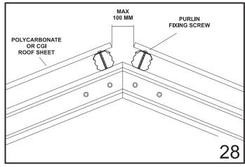
Crest fix CGI with 12x35mm roofing screws or polycarbonate sheeting with 12x45mm screws with polycarbonate washers. Sheets are fastened using five screws per sheet for end spans and three per sheet for internal spans. At the hip rafters and collar tie, sheets can be pan fixed with 10x16mm hex head self drilling screws.
