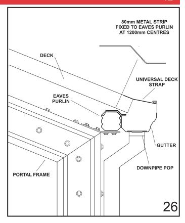
Construct two 70mm downpipe offsets from the downpipe lengths supplied and attach to the downpipe pop with rivets. Waterproof rivets with silicone. Fasten the downpipes with straps to the adjoining column.
