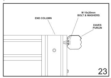
For rear attached units, fix the other end of the eaves purlin to the end of the rear attachment purlin as detailed in section 5.2.1.
