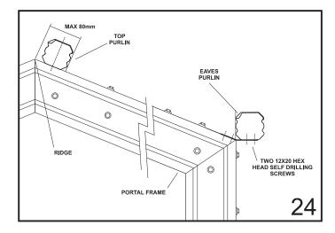
Where purlins are continuous over rafters, they are fixed in position using 14x95 hex head self drilling screws. If it is necessary for purlins to be broken over standard gable frames (ie, purlins continue in the same direction past a join) a 68mm in-line purlin connector is used (Figure 25).
