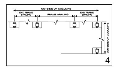
The end frame spacing, gives the centreline spacing between the rectangular end portal frame and the internal gable portal frame. Where more than two internal portal frames are required, space at the frame spacing dimensions specified on the drawings supplied.
