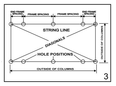
Tie string lines between the stakes to ensure the footings are in line. Check the dimensions and diagonals for squareness.
