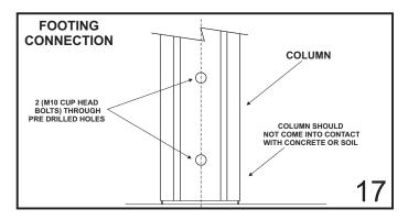
Bolt the footing plates to the chemical anchors installed earlier (refer Section 3.2).
