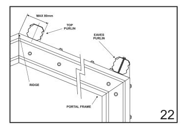
Where purlins are continuous over rafters they are fixed in position using 14x95 hex head self drilling screws. If it is necessary for purlins to be broken over standard gable frames (ie, purlins continue in the same direction past a join) a 68mm in-line purlin connector is used (Figure 23).
