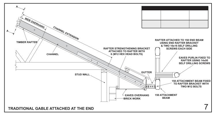
**Note:** Do not over tighten bolts as this can lead to a visible indentation due to the high gloss nature of the material. Refer to figure 8 for fixing spacers.
