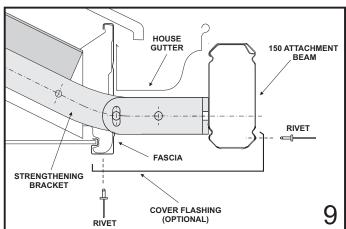
**Note:** It is the builders responsibility to ensure the existing rafters and fascia are adequately reinforced and strengthened to accommodate any additional attached structure. The reinforcing method must be approved by the appropriate council or engineer.
