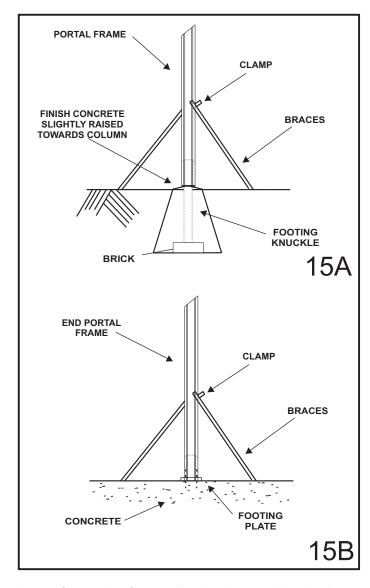
Locate frames in rafter to valley brackets and check column base is at the ground surface and the clear opening between the column and 150 attachment beam is correct. Finally and most importantly check that the columns are vertical.
