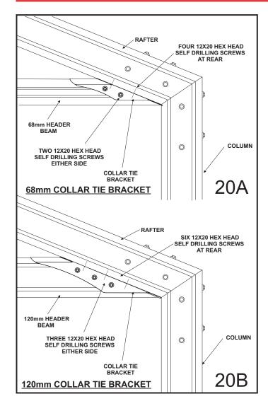
For a side attached Traditional Gable, on the attachment beam side, attach a collar tie bracket to the rafter to valley bracket using three 12x20 hex head self drilling screws at the rear. Fasten the header beam to the bracket using two 12x20 hex head self drilling screws each side (Figure 21).
