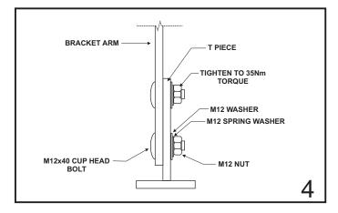
Insert the bracket through the fascia and fix with the channel(s) to the house rafter using M12 hex head bolts through the existing holes in the bracket and further up the channel(s) (Figure 6). Adjust the T piece so it is horizontal and has the appropriate extension past the fascia to allow for fixing of the attachment beam. T piece connection bolts are to be tightened to a minimum 35Nm torque.
